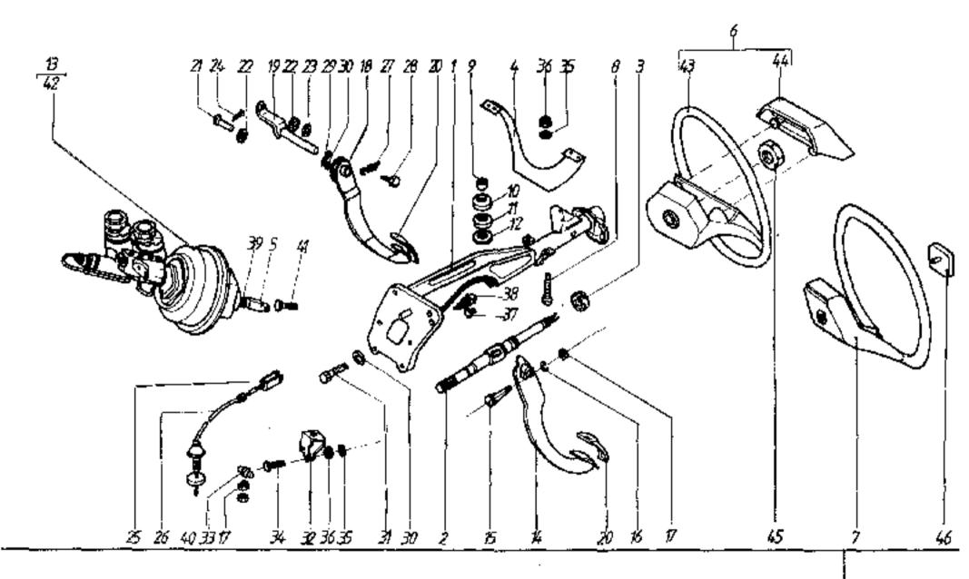
MONTAJ PEDALIER SI COL DIRECTIE STG. STEERING COLUMN AND PEDALS LH MONTAGE PEDALIER ET COLLONNE DE DIRECTION 6,
